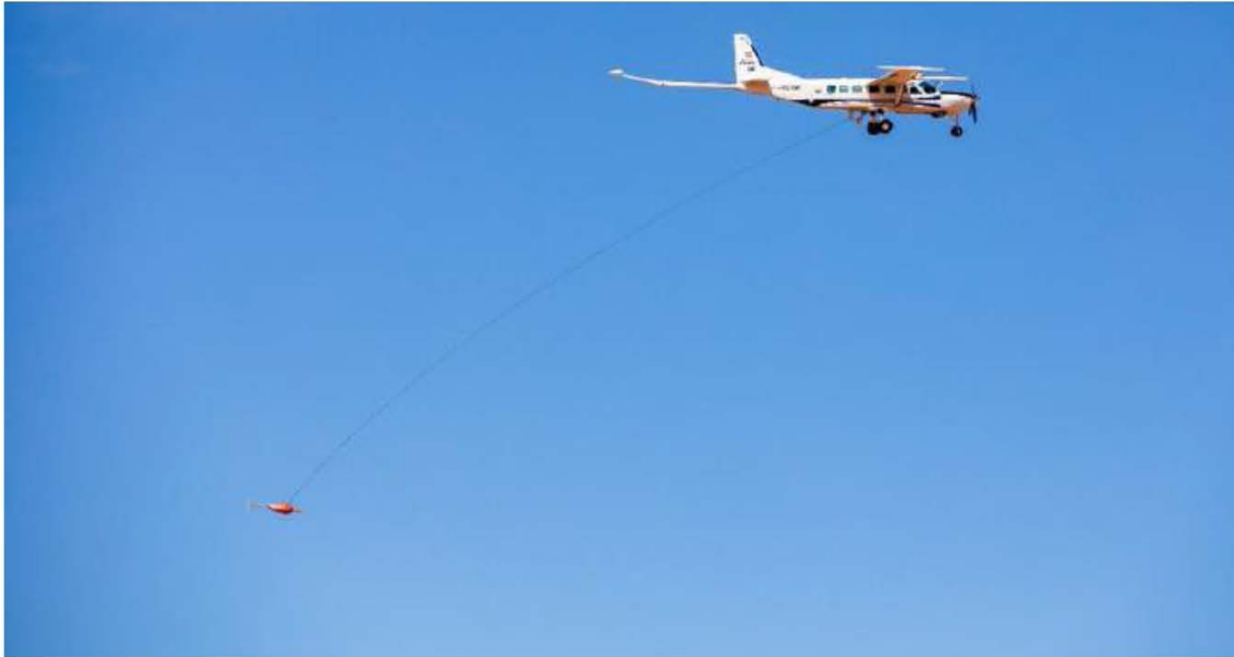
Figure 2 Example of Xcalibur fixed wing aircraft with receiver for AEM surveys.
